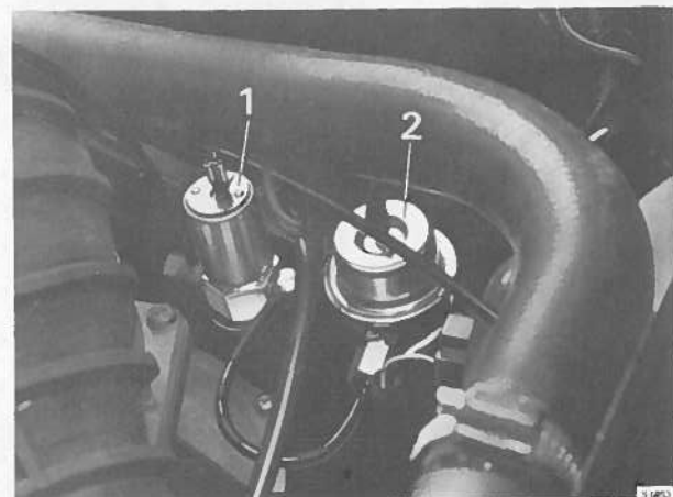
Solenoid switch and pressure regulator
