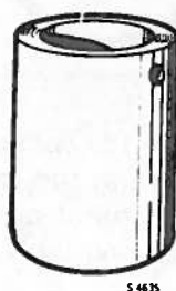
83 90 544 Dolly for removal of shaft from impeller
