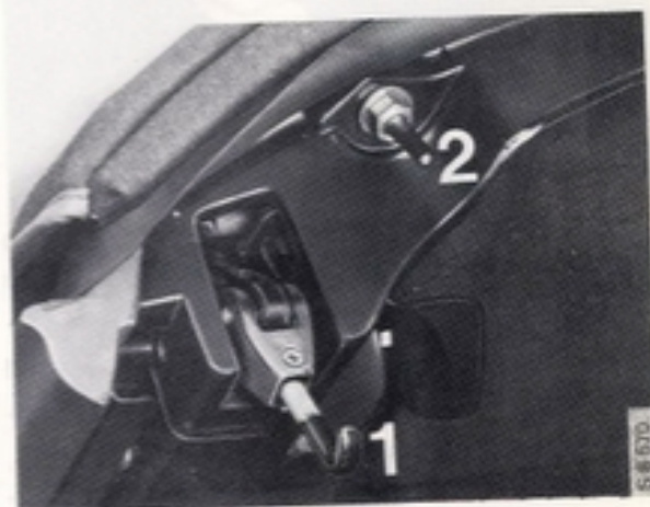
1 Hook, adjustment in height 2 Pin, adjustment, sideways
