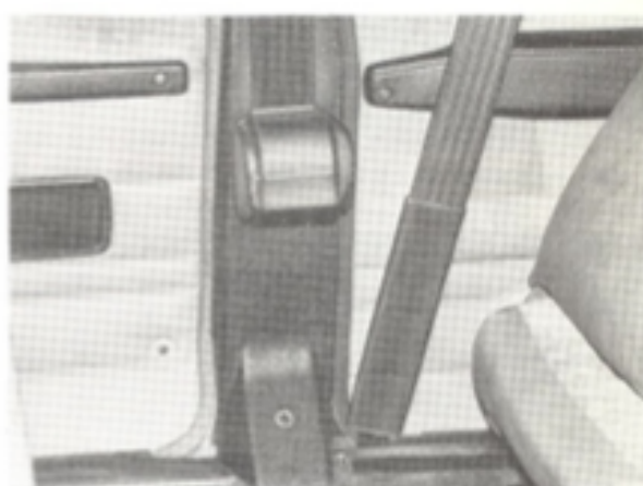
Front seat belt anchorage, 4- and 5-door cars as from 1981 models
