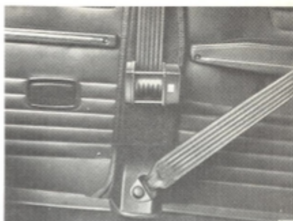
Front seat belt anchorage point in 5-door 1979-1980 models
