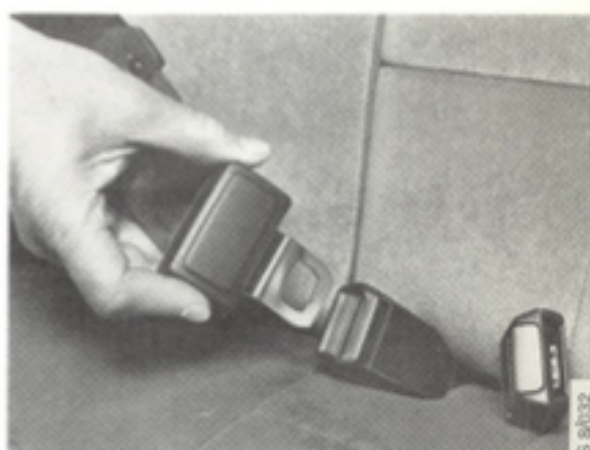
Buckle lock, rear seat belt, as from 1983 models
