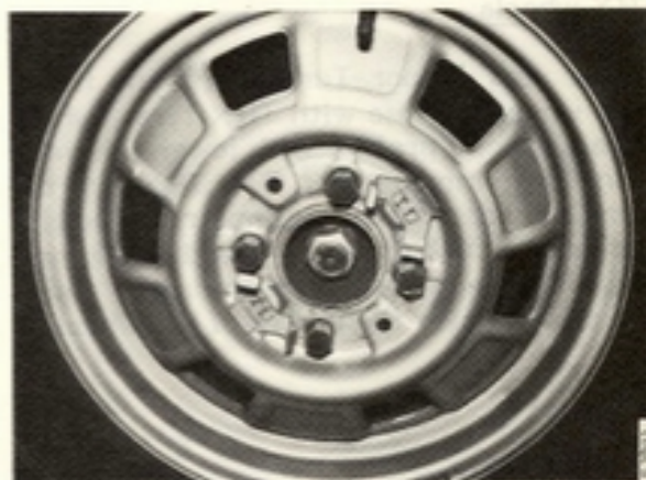
Hub cap clips, as from 1982 models
