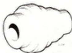
89 96 241 (A2) Drift, outer rings in rear wheel hubs
