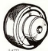
89 96 068 (A2) Drift, front wheel bearing in steering knuckle housing.
