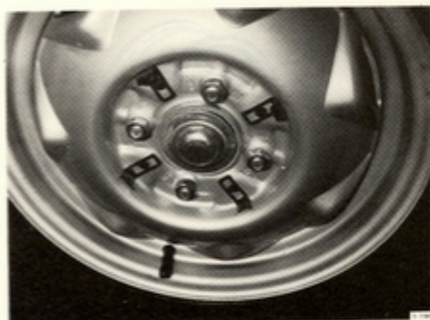
Hub cap clips, models 1979, 1980 and 1981
