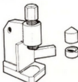
89 95 920 (A3) Tool, removal and installation of wheel studs
