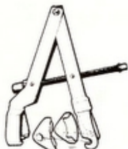
85 95 839 (A3) Spring compression tool, removal and installation of front coil spring
