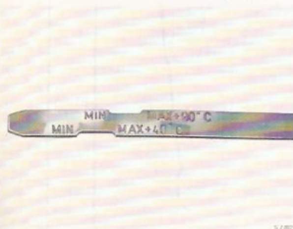
Dipstick, automatic transmission, type 37
